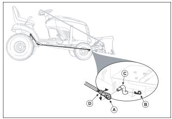
Figure 15. Lower Control Arm Installation
